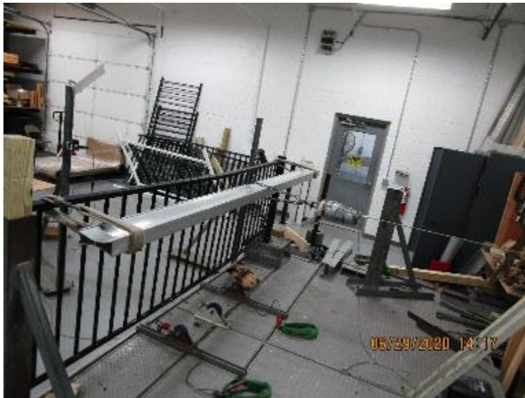
Photo No. 6 Concentrated Load Test at Ends of Rail (Brackets)
