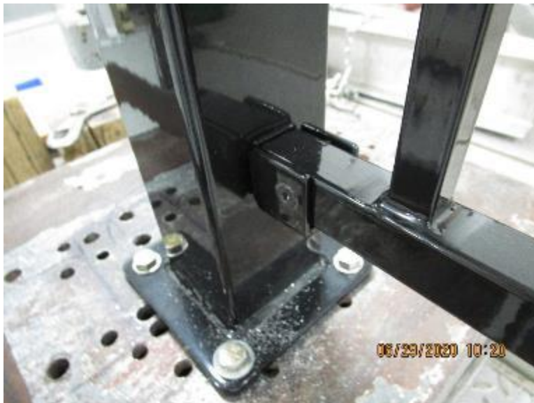
Photo No. 7 Bottom Rail Bracket and Post Mount Connection
