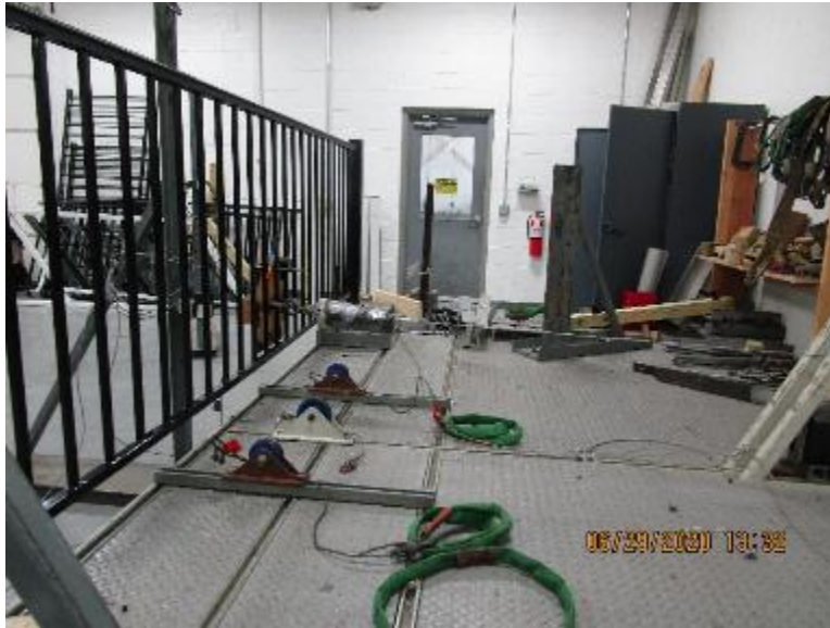
Photo No. 4 In-Fill Load Test at Bottom of Two Pickets
