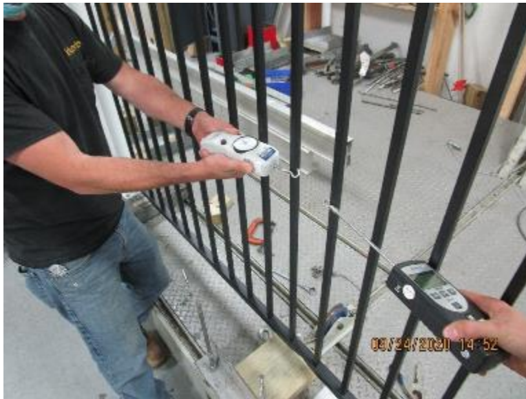
Photo No. 7 23 lb Test on Adjacent Pickets
