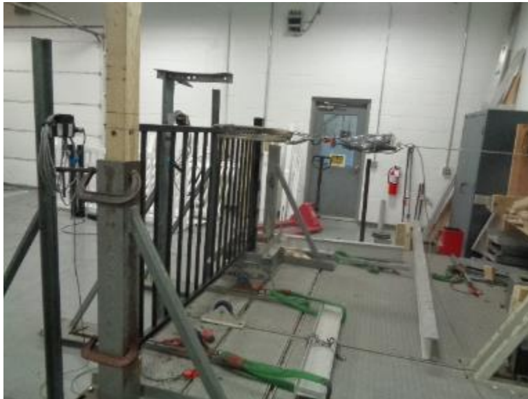
Photo No. 7 Horizontal Concentrated Load Test at Mid-Span of Top Rail
