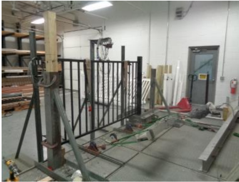
Photo No. 6 Vertical Uniform Load Test on Top Rail
