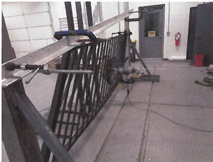
Photo No. 2 In-Fill Load Test at Center of Two Pickets
