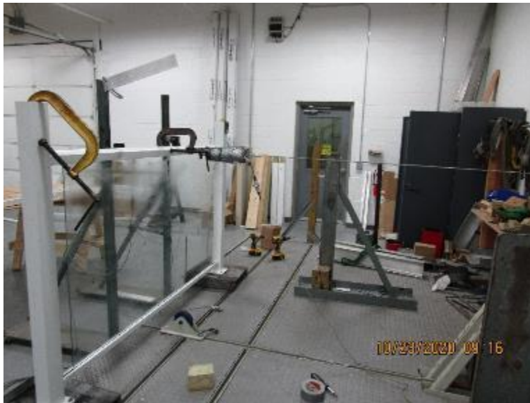
Photo No. 5 Concentrated Load Test at Midspan of Top Rail
