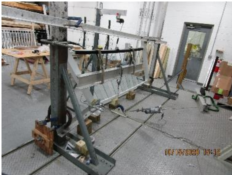
Photo No. 4 Vertical Uniform Test on Top Rail
