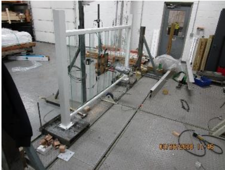
Photo No. 1 In-Fill Load Test at Center of Two Balustrades
