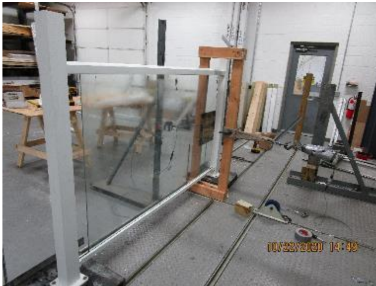
Photo No. 3 In-Fill Load Test at Center of Edge of Glass Panel
